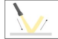
Left: Light travelling and reflecting off a smooth surface
